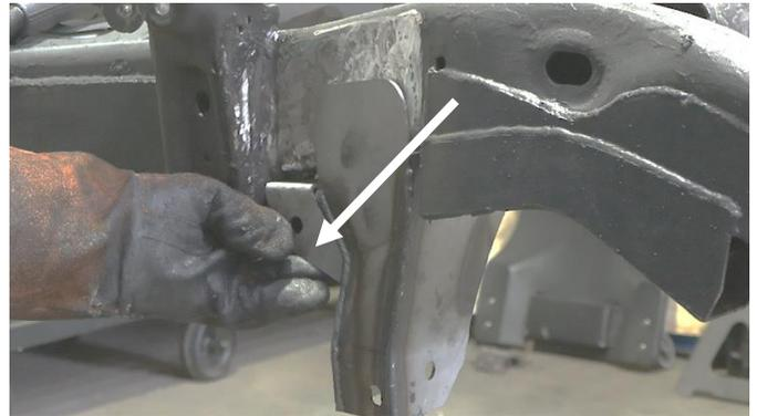
Once aligned, tac weld the support bracket to the track bar bracket before welding the parts on fully. Weld 100% around all edges.
