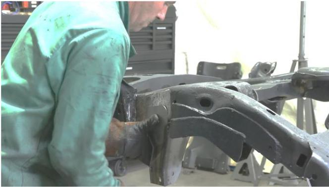
Following proper welding procedure, tac weld the track bar bracket onto the frame.
