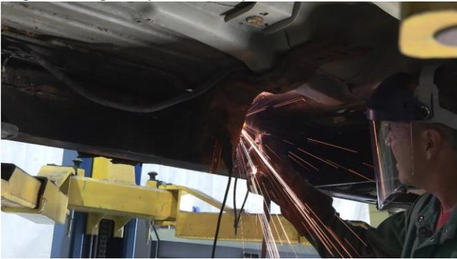
Grind and clean the frame free of rust and debris, revealing bare metal. Followed by coating the work area with a weld through primer to prevent against further rust development.
