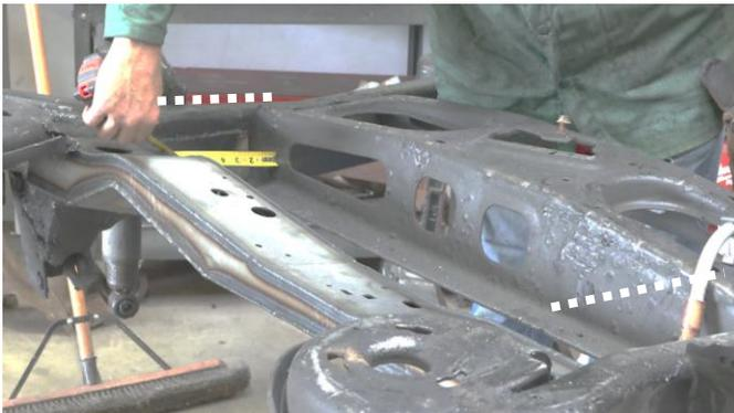
Finish tac welding the part onto the frame before welding it on fully. Weld 100% around all edges.
