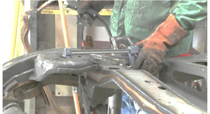
Using a tape measure, measure the distance between the track bar crossmember and the spare tire crossmember, making sure the distance between them is the same on both ends.
