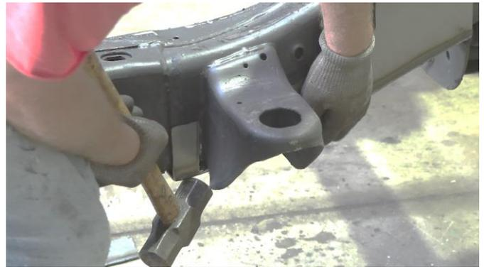
Once in place, mark each end of the frame section using a paint marker.
