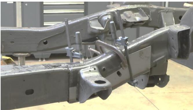
Following proper welding procedures, tac weld your front frame section into place before welding the part on fully. Weld 100% around all edges.
