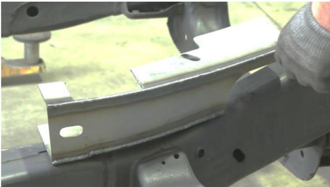
Slide the front frame section onto the frame using a hammer to tap it into place. Use the frame holes to help with the alignment.
