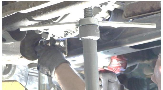
Insert a bolt on each end of the transmission crossmember to hold it in place. Then, lower your jack stand supporting the crossmember.
