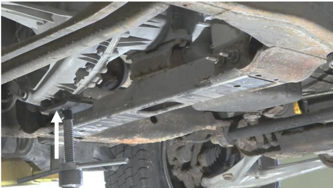
With a 5/8" socket, remove the two bolts in the center.
