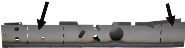
Draw a line approximately 5/16" to a 1/2 inch above the bottom of the frame and cut along it.
