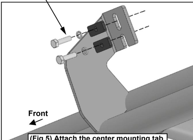
(Fig 5) Attach the center mounting tab on the Armor to the center location
