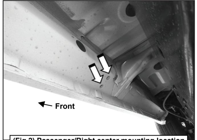
(Fig 2) Passenger/Right center mounting location
