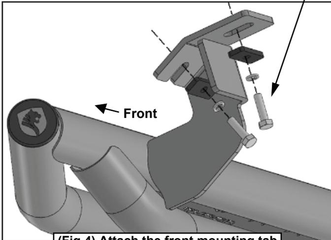
(Fig 4) Attach the front mounting tab on the Armor to the front location
