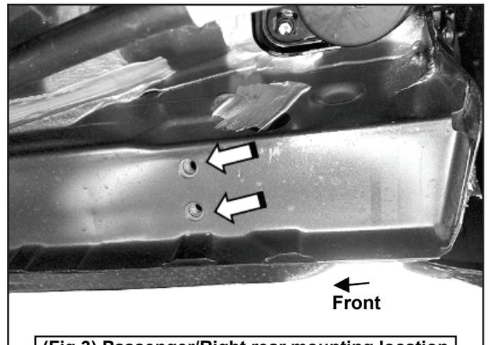
(Fig 3) Passenger/Right rear mounting location
