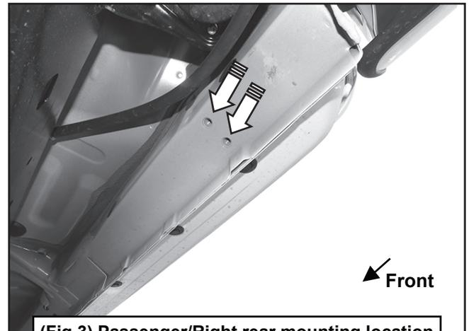
(Fig 3) Passenger/Right rear mounting location
