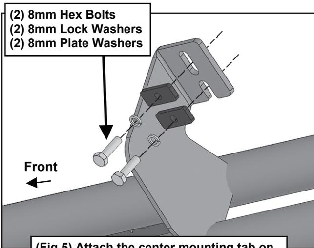
(Fig 5) Attach the center mounting tab on the Tyger Armor to the center location
