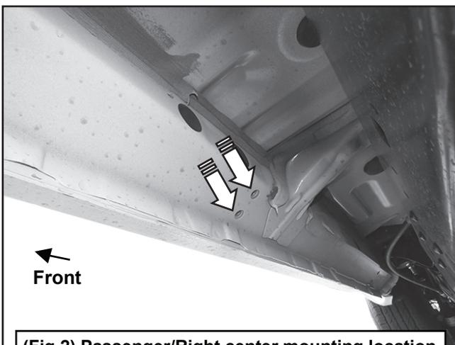
(Fig 2) Passenger/Right center mounting location
