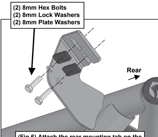
(Fig 6) Attach the rear mounting tab on the Tyger Armor to the rear location
