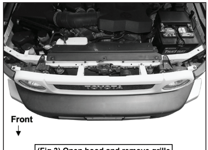
(Fig 3) Open hood and remove grille
