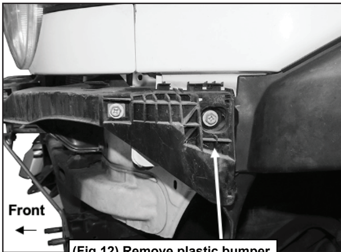
(Fig 12) Remove plastic bumper clip (driver/left side pictured)
