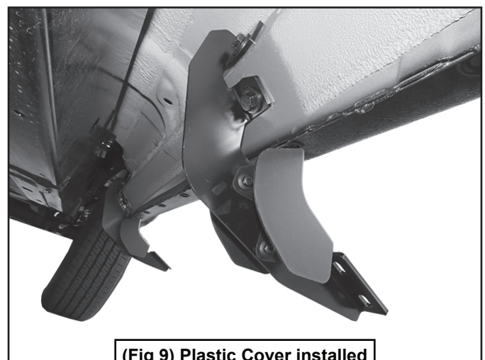
(Fig 9) Plastic Cover installed
