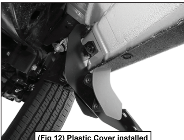
(Fig 12) Plastic Cover installed
