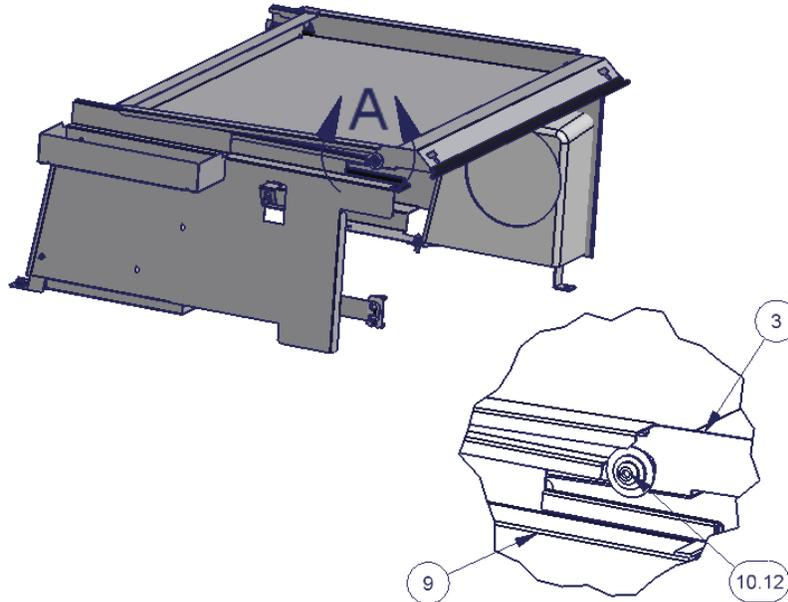
23. Check the seal between the vehicle rear door and the lid. Close the top rear window and check the clearance with the lid. Loosen the mounting hardware and maneuver the enclosure so there is a good seal and clearance between the top rear window if necessary.
