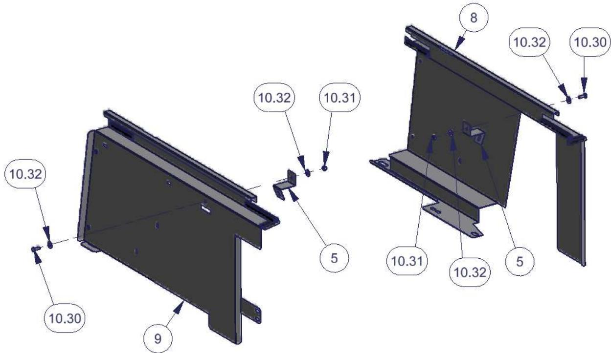
7. Install the #7 trays to both sides #8 and #9 using the illustrated hardware. (See Figure 3)
