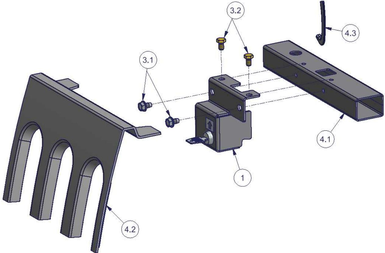
**Optional #091 Dust Cover installation & Cam orientation**
