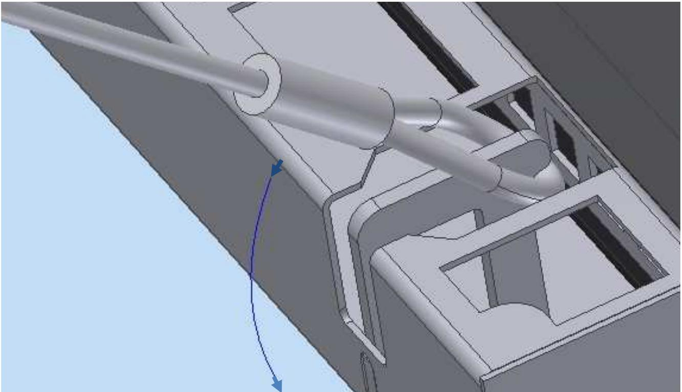
2. Rotate lanyard down over the post.
