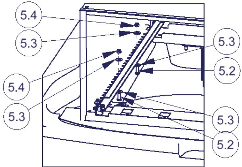
10. Adjust all three apron pieces to minimize the gaps around the enclosure, then using (4) #5.2 Bolts, (4) #5.4 Nuts, and (8) #5.3 Flat Washers attach the #7 Side Aprons to the enclosure. (See Figure 8) NOTE: The mounting holes in the enclosure and aprons allow for some variability, but in some situations new holes in the aprons may need to be marked and drilled to minimize gaps or prevent overlapping of the apron components.
