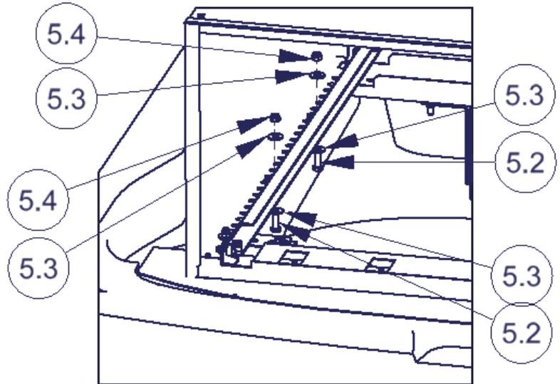
10. Adjust all three apron pieces to minimize the gaps around the enclosure, then using (4) #5.2 Bolts, (4) #5.4 Nuts, and (8) #5.3 Flat Washers attach the #7 Side Aprons to the enclosure. (See Figure 8) NOTE: The mounting holes in the enclosure and aprons allow for some variability, but in some situations new holes in the aprons may need to be marked and drilled to minimize gaps or prevent overlapping of the apron components.
