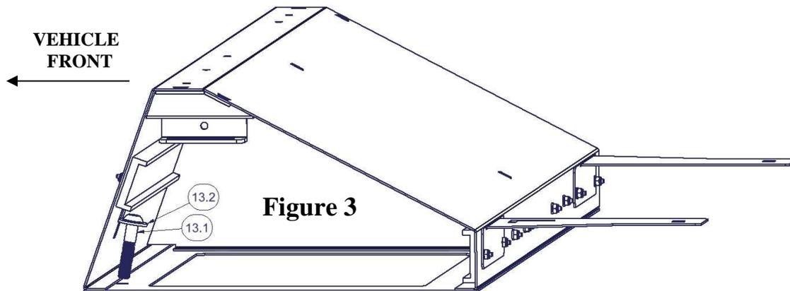
13. Center the enclosure over all the mounting points and tighten the mounting hardware.
