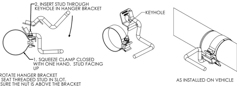
3. Slide the **Hang Tight™ Hanger Clamp Assembly** over the **Extension Pipe** and install the **Muffler** onto the **Extension Pipe**. Install the **Hang Tight™ Hanger** into the existing rubber insulator. Refer to Figure 5.
