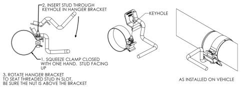
2. Using the **2.5" Clamp**, install the reduced end of the **Extension Pipe** over the factory exhaust system behind the "Y" pipe. Install the **Hang Tight™ Hanger** Clamp assembly over the Extension pipe and into the factory rubber insulator. Install the Mid Pipe if required using a **3.0" Clamp**, see the chart below for pipe modifications. Cut the **Extension Pipe** if required.
