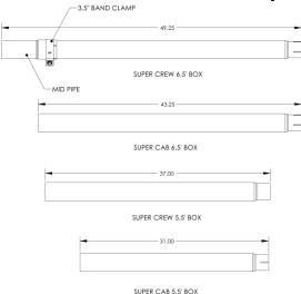
3. Using the **3" Clamps**, install the **Muffler** onto the **Extension Pipe** (or **Mid Pipe** if required), and install the **Over Axle Pipe** into the opposite end of the **Muffler**. Install the **Over Axle Pipe** hanger into the factory rubber insulator located above the rear of the **Muffler**.
