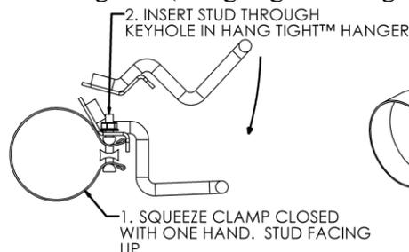
3. ROTATE HANG TIGHT™ HANGER TO SEAT THREADED STUD IN SLOT. BE SURE THE NUT IS ABOVE THE BRACKET
