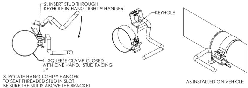
4. Install the hanger assembly from step 3 loosely to the **Extension Pipe** (or **Front Pipe** if the **Extension Pipe** is not required) and place the hanger into the existing rubber insulator.
