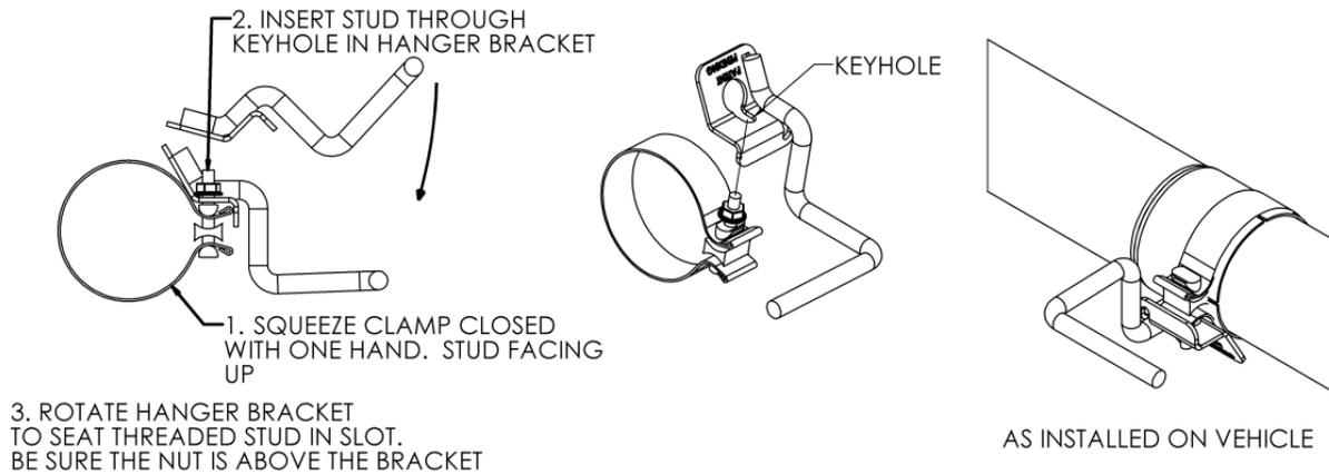
5. Slide the **3" Hang Tight™ Clamp** over the outlet side of the **Muffler**. Position the **Turn Down** and loosely attach it to the **Muffler**. Install the **3" Hang Tight™** into the existing rubber insulator.
