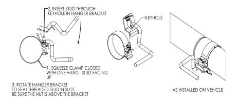
3. Install the Hang Tight™ Hanger assembly over the Extension Pipe and into the OEM rubber isolator located on the frame near the end of the Extension Pipe.
