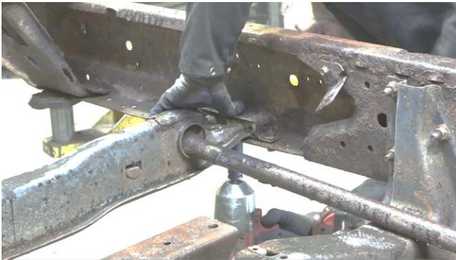
Then, remove the two bolts retaining the crossmembers bracket with a 15mm socket and 18mm wrench.
