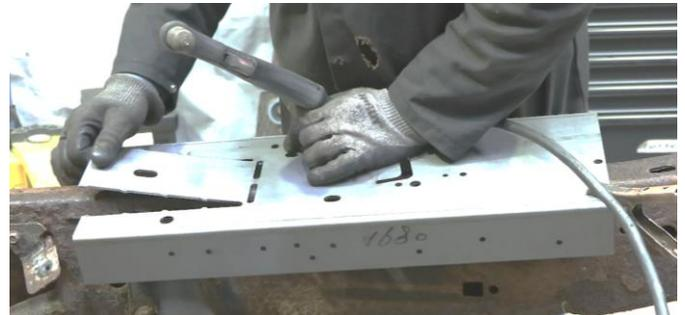
Slide your center frame section onto the frame using the frame holes to help with the alignment. Tap it into place using a hammer.
