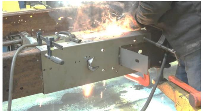
Then, clamp your plate against the frame using a c-clamp, followed by welding the plate into place.
