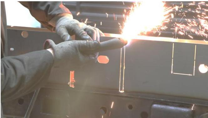
After removing the necessary plates, we will need to cut and remove the bottom of the frame where your mid frame section will sit. To do this, hold your mid frame section up to the frame and mark off its coverage. Then, remove approximately half an inch off the bottom of the frame.
