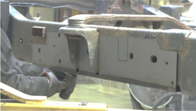
Following proper welding procedures, tack weld your mid frame section onto the frame before welding it on fully. Weld 100% around all edges.
