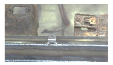
After welding the brackets onto your replacement crossmember, cut out the factory crossmember and any obstructions in the work area.
