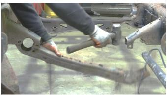
After removing the crossmember, clean the area free of rust and debris, revealing bare metal.
