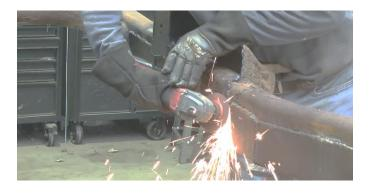
Next, hold the replacement forward gas tank crossmember up to the frame and mark off the section of the body mount that needs to be removed for the crossmember to fit properly. We recommend measuring twice to ensure that you're cutting the right amount of material. Then, cut off the marked section of your body mount.
