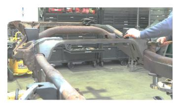
Once you have your crossmember in place, follow proper welding procedures and tac weld your crossmember to the frame. Then, weld the part on fully. Weld 100% around all edges.
