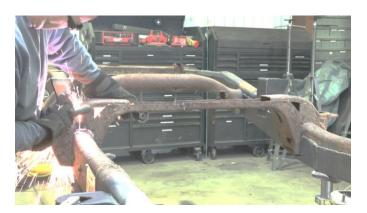
After removing your crossmember, grind the frame free of rust and debris, revealing bare metal.
