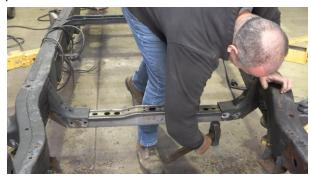
**NOTE:** The large circular holes on the top of your crossmember should be facing straight up.
